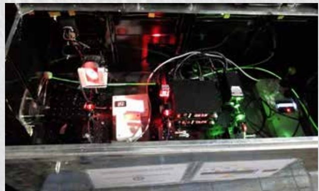
Figure 3. Photographs of the solar-powered artificial light coupling system installed at Jhanjra coal mine (left). The lasers and the optical coupler assembly used for illumination are shown (right).
