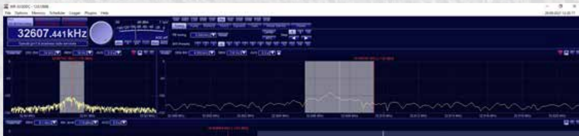
Fig. 14 Measured signal level when transmitter at the 4 th pillar (approx. 120 meters).
