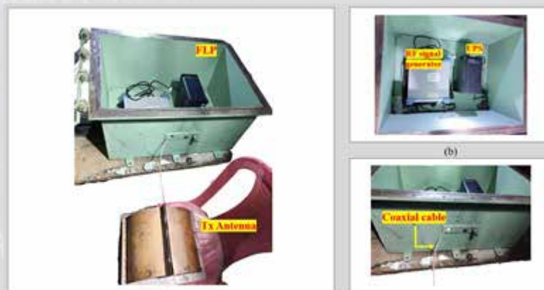
Fig. 10 Transmitter setup for the underground station (the photograph is taken outside mine before installation inside mine) (a) Complete transmitter setup with FLP (b) FLP containing RF signal generator and power supply (UPS) (c) Side view of FLP showing the cable.
