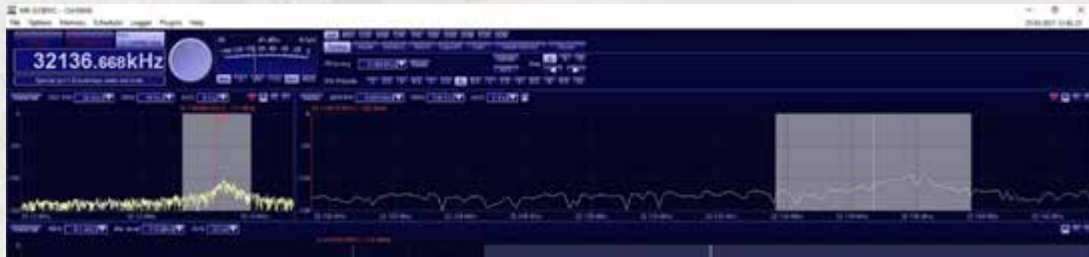
Fig. 13 Measured signal level when transmitter at the 3 rd pillar (approx. 90 meters).
