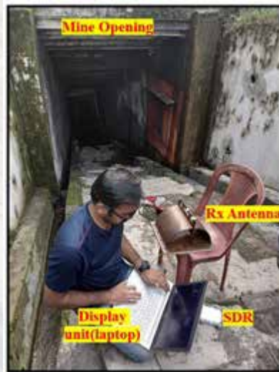
Fig. 11 Receiver setup for a surface station
